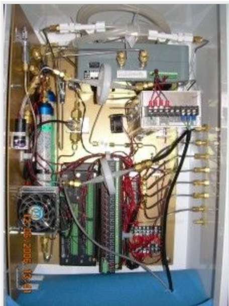
CO 2 measurement system using a single-cell NDIR-based analyzer.
